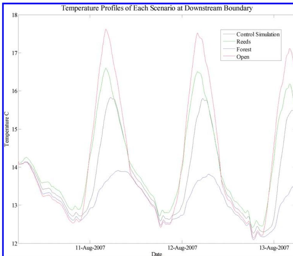
FIGURE 3. Modeled stream temperature outputs at the downstream boundary of each vegetation cover scenario relative to the calibrated model simulation including the three sections of different vegetation type.
