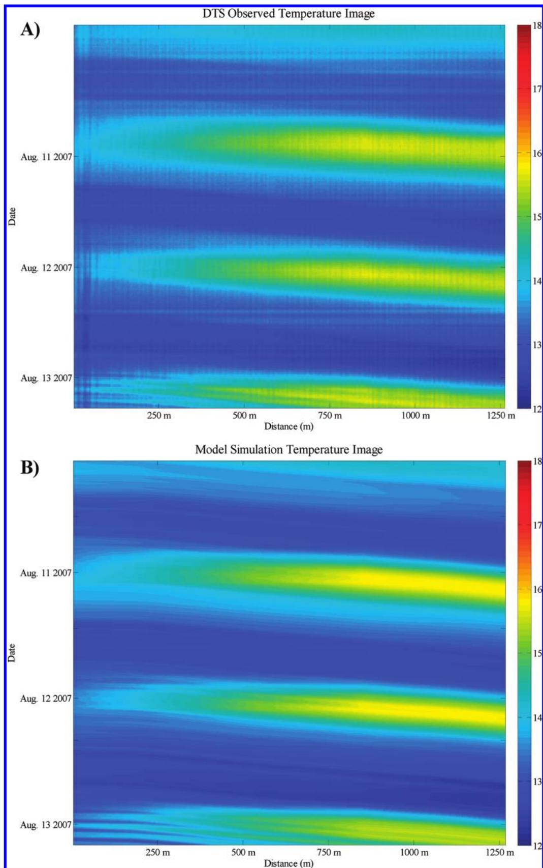
**FIGURE 2. (A) DTS observed temperature over the length of the stream and the duration of the experiment and (B) control simulation temperature over the same time frame. The visible temperature striations on August 13 are a result of upstream pumping. The color bar represents temperature in degrees Celsius.**
